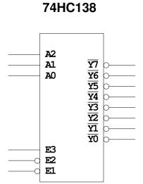
When E3 high, E2 and E1 low, one of the outputs of the 74138 will go low A2, A1, A0 determine which output will be low.
