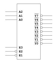
Want to select external device when E is high -- Connect E to E3
