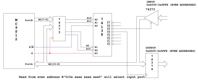
Write to even address B"010x xxxx xxxx xxx0" will latch data in output port
