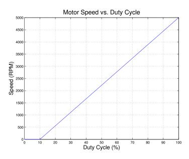
The motor doesn't start rotating until it is driven with a 10% duty cycle, after which it will increase speed linearly with the increase in duty cycle.
