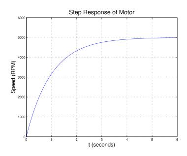
We will control the motor by adjusting the duty cycle with the MC9S12. We will do this by measuring the speed and updating the duty cycle on a regular basis. Let's do the adjustments once every 8 ms. This means that we will adjust the duty cycle, wait for 8 ms to find the new speed, then adjust the duty cycle again. How much change in speed will there be in 8 ms? The motor behaves like a single time constant system, so the equation for the speed as a function of time is:
