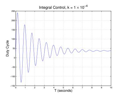
To get this oscillating response, the duty cycle must go to over 100%, and below 0%, which is clearly impossible. To get the response we expect in the lab, we need to limit the duty cycle to remain between 20% and 100%. Thus, we change our simulation to be:
