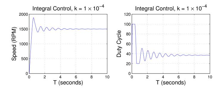
In your program for Lab 5, you will use a Real Time Interrupt with an 8 ms period. In the RTI interrupt service routine, you will measure the speed, and set the duty cycle based on the measured speed. Your ISR will look something like this:
