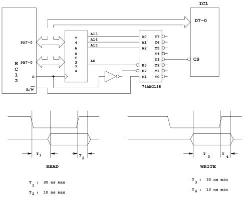
(a) Is IC1 an input or an output port? Explain.
