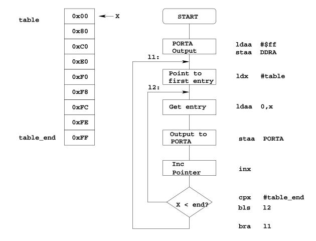
Flowchart to display a pattern of lights on a set of LEDs
