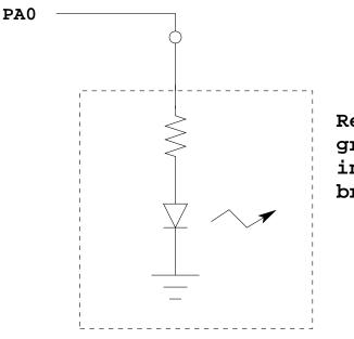
Resistor, LED, and ground connected internally inside breadboard
