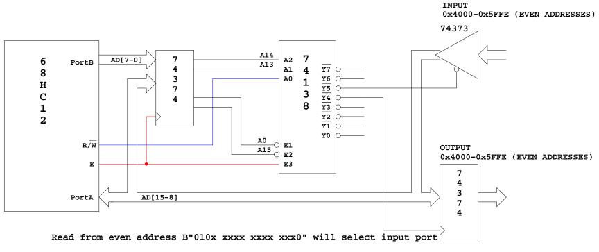
Write to even address B"010x xxxx xxx0" will latch data in output port
