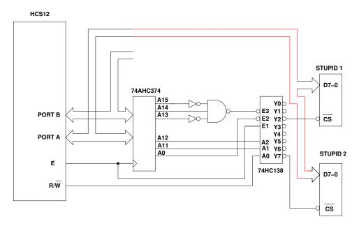
(a) What range of addresses will select STUPID 1 chip? Is it an input chip or an output chip.
