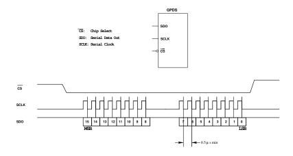
(a) Sketch how you would connect the GPDS to an HCS12. That is, show where the SCLK, SD0 and  $\overline{\text{CS}}$  will connect to the HCS12.
