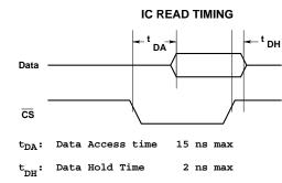
i. How long is it from the time E goes high until  $\overline{CS}$  goes low? (Assume there are no E-clock stretches.)
