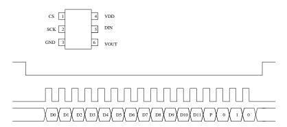
(a) Sketch how you would connect the D/A to a 9S12. That is, show where the SCK, DIN and  $\overline{\text{CS}}$  will connect to the HCS12.
