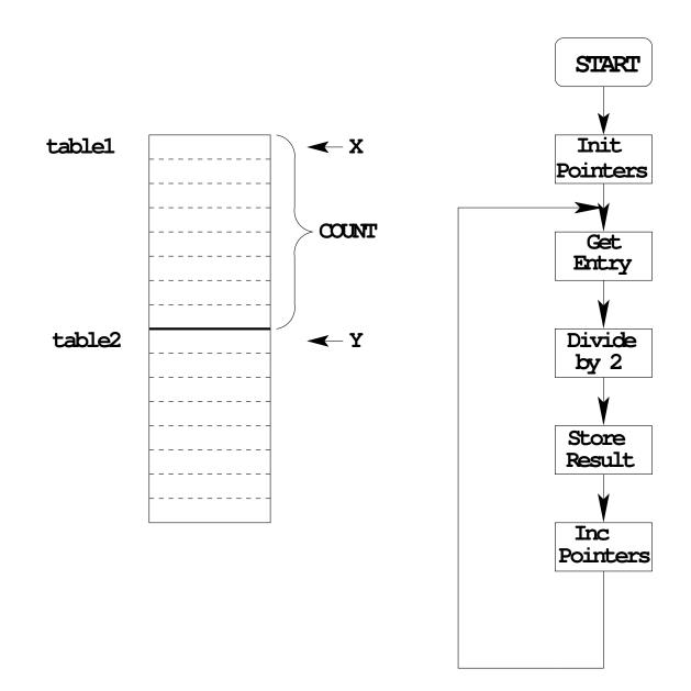
6. Need a way to determine when we reach the end of the table. One way: Use a counter (say, register A) to keep track of how many elements we have processed.
