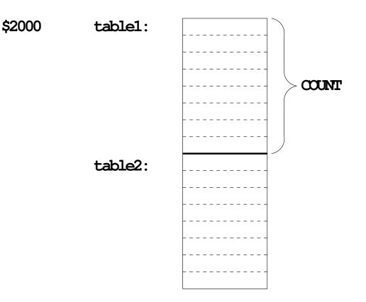
4. Strategy: Because we are using a table of data, we will need pointers to each table so we can keep track of which table element we are working on.
