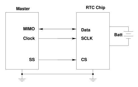
When used as a master in bidirectional mode, the Master Out Slave In pin becomes the Master Out Master In Pin
