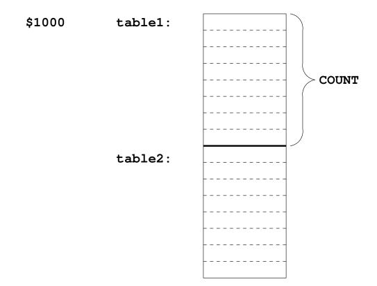
4. Strategy: Because we are using a table of data, we will need pointers to each table so we can keep track of which table element we are working on.
