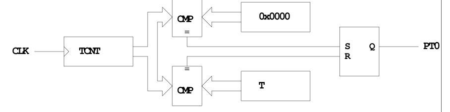
When TCNT = 0x0000, the output goes high When TCNT = T, the output goes low
