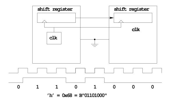
Need 3 wires to transmit 1 bit at a time
