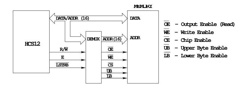
HCS12 has 16-bit address and 16-bit data buses
