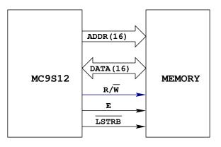
READ: MC9S12 puts address on address bus brings R/W high Memory puts data on data bus HC12 latches data on falling edge of E clock
