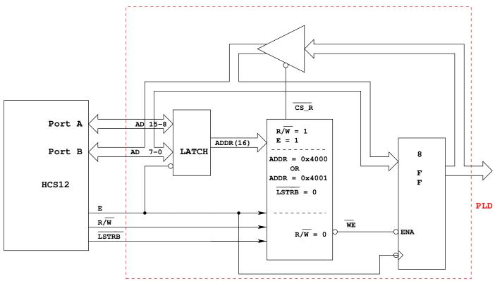
Writing to address 0x4001 (ADDR = 0x4000 or 0x4001, LSTRB low, R/W low) will bring WE low. On the high-to-low transition of E with WE low, the data into the flip-flops
