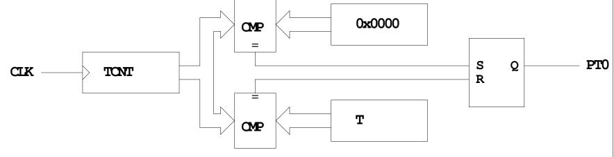
When TCNT = 0x0000, the output goes high When TCNT = T, the output goes low
