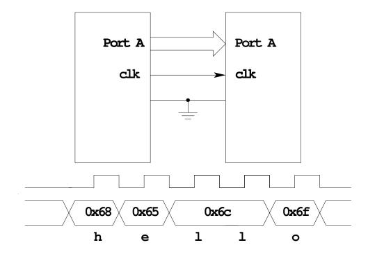
Need 10 wires to transmit 8 bits of data
