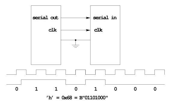
Need 3 wires to transmit 1 bit at a time
