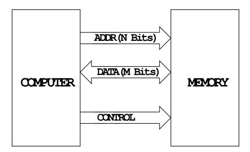
Computer with N bit address bus can access  $2^{N}$  bytes of data
