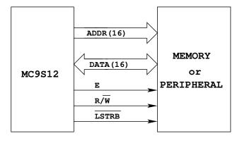
MC9S12 has 16 bit address bus - can access 65536 bytes
