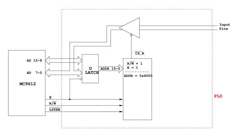
Reading from address 0x4000 (ADDR = 0x4000, R/W high, E high) will bring CS\_R low This will drive the data from the input pins onto the data bus The MC9S12 will read the data on the input pins on the high-to-low transition of the E-clock
