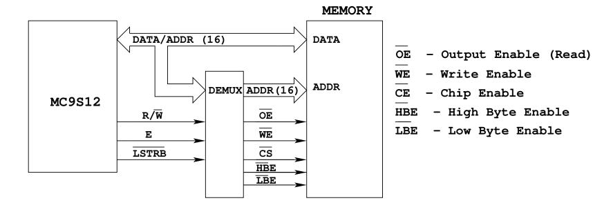
MC9S12 has 16-bit address and 16-bit data buses
