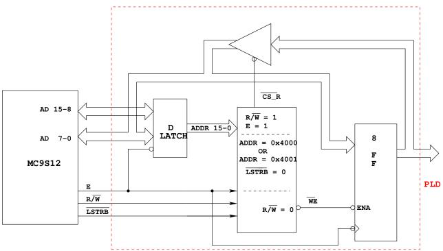
Writing to address 0x4001 (ADDR = 0x4000 or 0x4001, LSTRB low, R/W low) will bring WE low. On the high-to-low transition of E with WE low, the data is latched into the flip-flops
