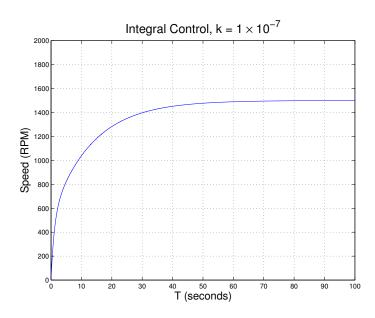
With this value of k, it will take about 1 minute for the motor to get to the desired speed.
