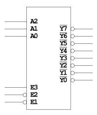
When E3 high, E2 and E1 low, one of the outputs of the 74138 will go low A2, A1, A0 determine which output will be low.
