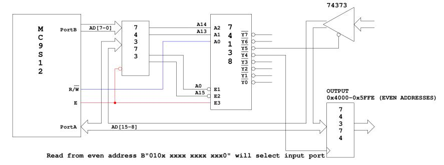
Write to even address B"010x xxxx xxxx xxx0" will latch data in output port
