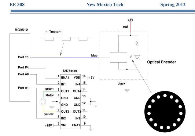
Figure 1: Using a PWM signal to adjust the speed of a motor.
