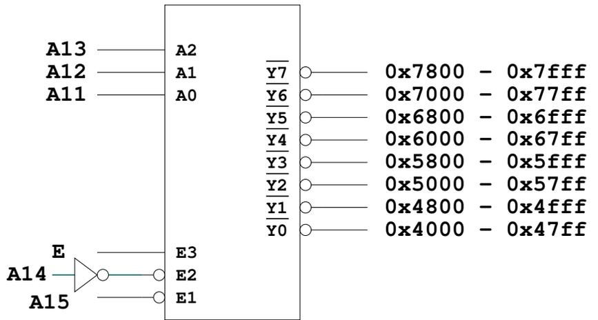
Nothing is mapped into memory spaces occupied by outputs Y2 through Y7
