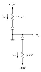
$V_O$  is connected directly to ground, so  $V_O = 0$  V.
