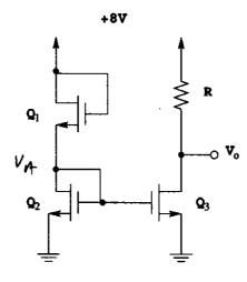
$$\begin{array}{l} Q_{1}+Q_{2} \quad id_{e_{A}}+ia_{a} \\ T_{b_{1}}=T_{b_{2}} \quad = ) \quad V_{GS_{1}}=V_{GS_{2}} \quad = ) \quad 8-V_{A}=V_{A}=) \quad V_{A}=4V \\ T_{b_{1}}= \quad \dot{z} \quad h_{n}'\left(\frac{W}{E}\right)\left(V_{GS_{1}}-V_{E_{1}}\right)z \quad \dot{z}\left(S_{\mu}A/v^{2}\right)\left(4v-2v\right)^{2} \\ \quad = \quad 2o_{\mu}A \end{array}$$
