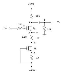
The MOSFET's are matched, and  $k'_n(W/L) = 2 \text{ mA/V}^2$ , and  $V_t = -2 \text{ V}$ . Ignore the output resistance  $r_o$ , and assume all capacitors are large (all AC signals are passed through, all DC signals are blocked).
