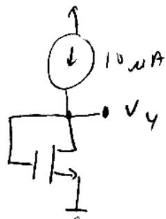
$$V_{DS} = V_{GS} > V_{GS} - V_t, \text{ so Q in saturation}$$
