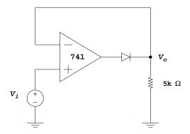
4. Substitute a 411 op amp for the 741. Compare the behavior of the two rectifiers at 2 kHz frequency. Why is the performance improved with the 411?
