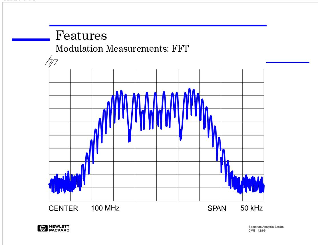
We've just seen how modulation frequency and AM depth of modulation measurements using a spectrum analyzer can be made in both the swept-frequency-domain and the FFT-frequency-domain. So why would you want to use the FFT function?
