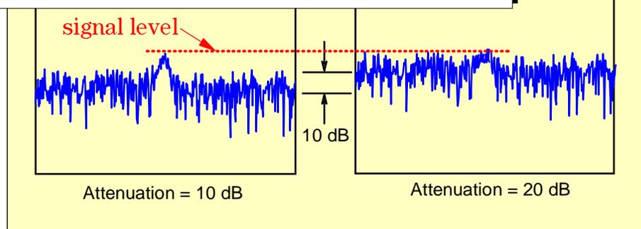
Signal-To-Noise Ratio Decreases as RF Input Attenuation is Increased
