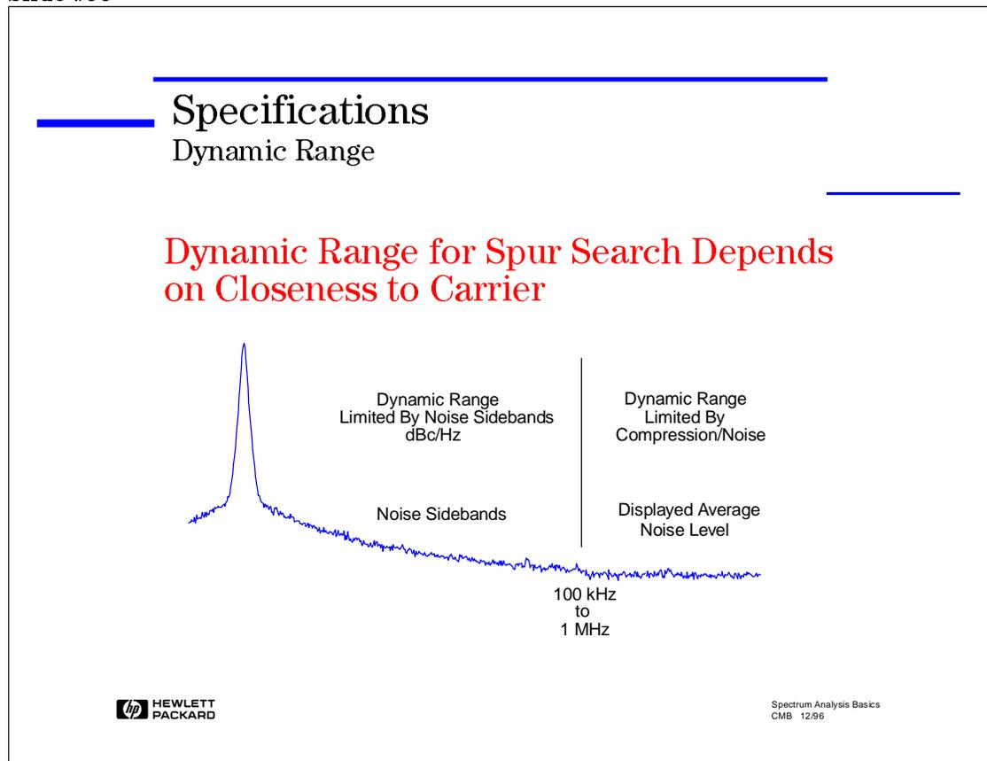
The final factor in dynamic range is the phase noise, or noise sidebands, on our spectrum analyzer LO.
