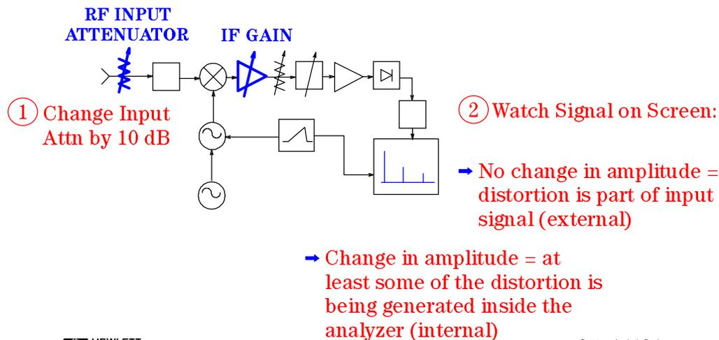
Before leaving this section on distortion, there is a test that should be done for all distortion measurements. The test is going to tell us whether or not what we are seeing on the screen is internally generated distortion, or distortion caused by the DUT.
