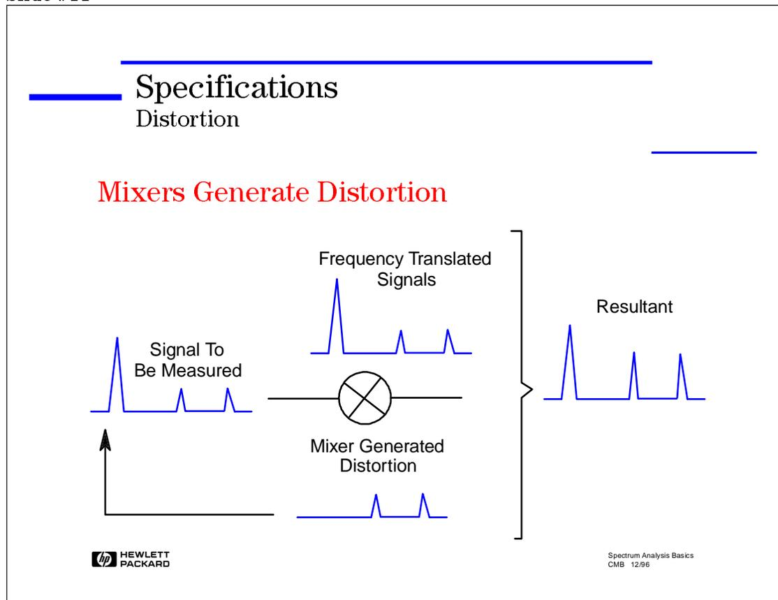
Although distortion measurements, such as third order intermodulation and harmonic distortion, are common measurements for characterizing devices, the spectrum analyzer itself will also produce distortion products, and potentially disturb your measurement.
