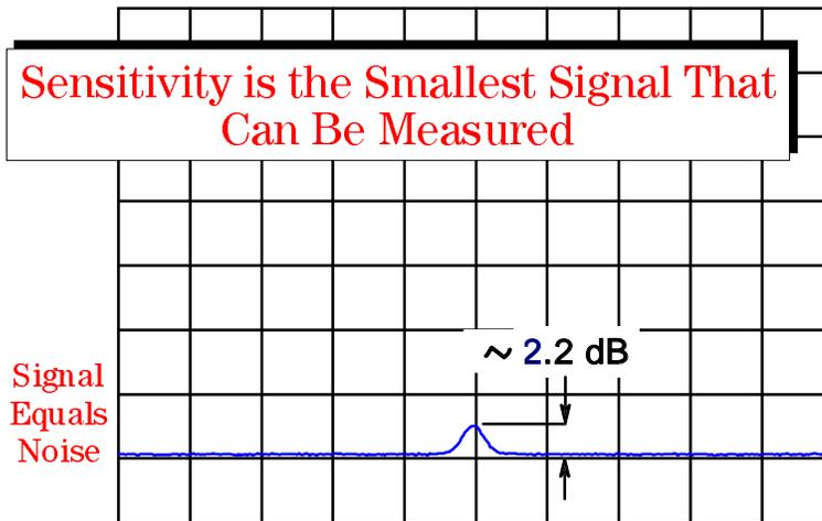
A signal whose level is equal to the displayed average noise level (DANL) will appear approximately as a 2.2 dB bump above the displayed average noise level. This is considered to be the minimum measurable signal level. However, you won't be able to see this signal unless you use video filtering to average the noise.
