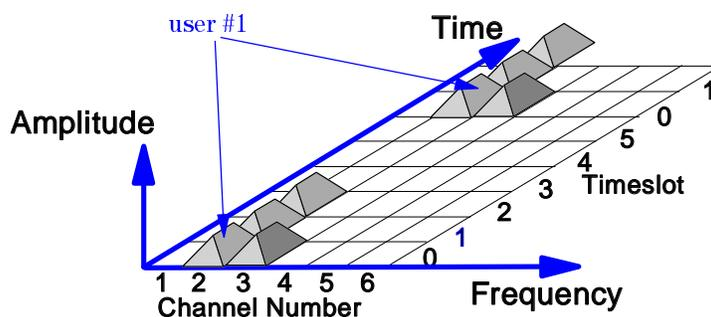
In order to explain the time-gating feature of a spectrum analyzer, we will use a digital communications application, Time-Division-Multiple-Access (TDMA). This is a common method used in communications in order to increase channel capacities in the same frequency bands. TDMA divides up the frequency channels into time slots, so that users can occupy the same frequency, but use different timeslots.
