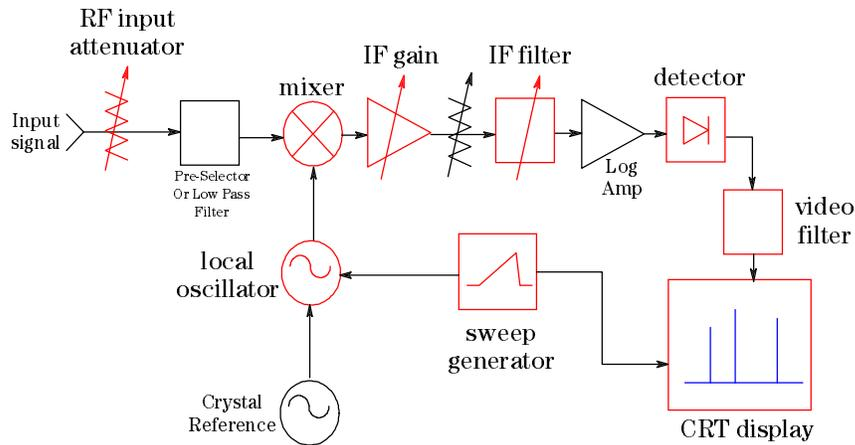
The major components in a spectrum analyzer are the RF input attenuator, mixer, IF (Intermediate Frequency) gain, IF filter, detector, video filter, local oscillator, sweep generator, and CRT display. Before we talk about how these pieces work together, let's get a fundamental understanding of each component individually.
