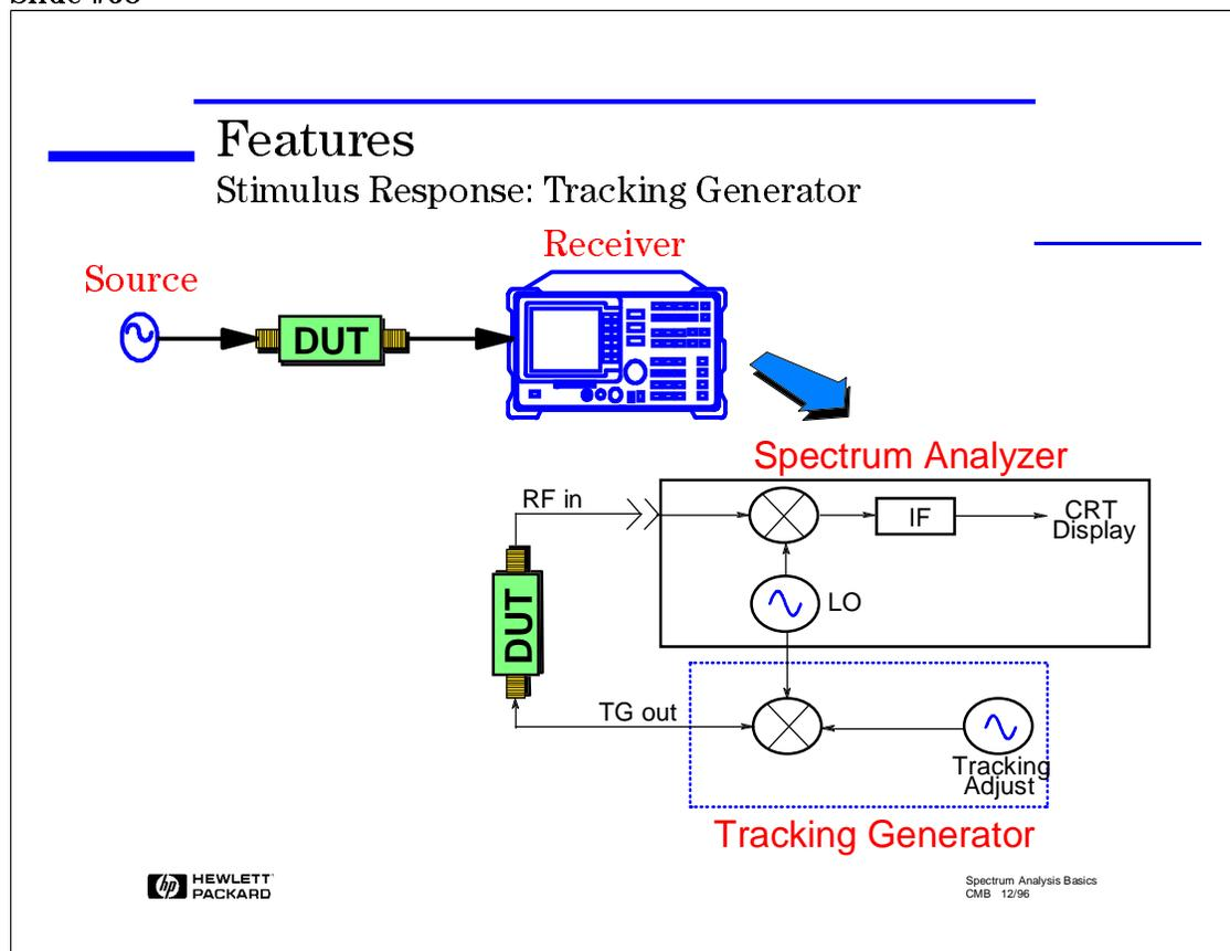
Stimulus response measurements, or network measurements, involve applying a signal to the input of our device/system and measuring the response at the output. Therefore, they require a source to stimulate the DUT and a receiver to analyze the transfer characteristics of the DUT. Common measurements include frequency response, return loss, conversion loss, and gain versus frequency.
