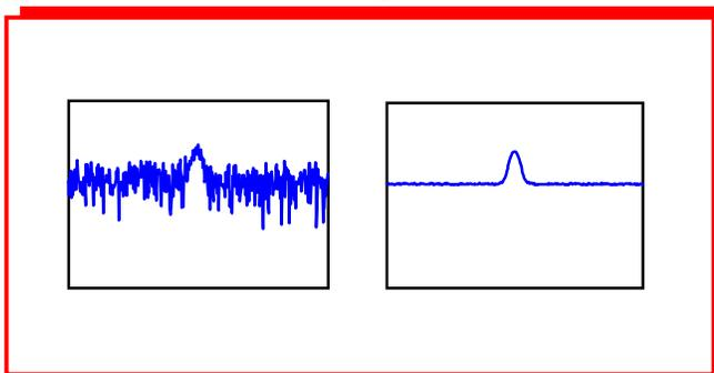
The video filter is a low-pass filter that is located after the envelope detector and before the ADC. This filter determines the bandwidth of the video amplifier, and is used to average or smooth the trace seen on the screen.
