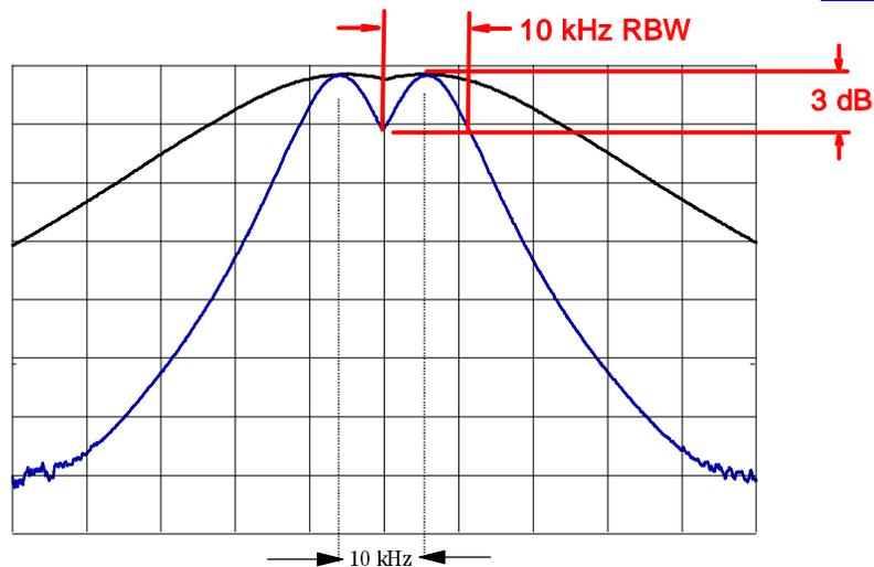
When measuring two signals of equal-amplitude, the value of the selected RBW tells us how close together they can be and still be distinguishable from one another (by a 3 dB 'dip'). For example, if two signals are 10 kHz apart, a 10 kHz RBW easily separates the responses. However, with wider RBWs, the two signals may appear as one.
