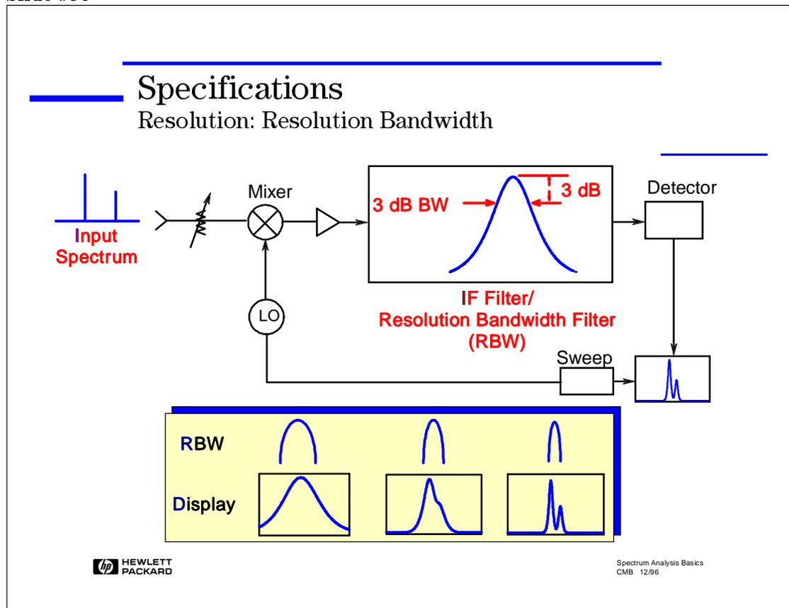
One of the first things to note is that a signal cannot be displayed as an infinitely narrow line. It has some width associated with it. This shape is the analyzer's tracing of its own IF filter shape as it tunes past a signal. Thus, if we change the filter bandwidth, we change the width of the displayed response. HP datasheets specify the 3 dB bandwidth. Some other manufacturers specify the 6 dB bandwidth.
