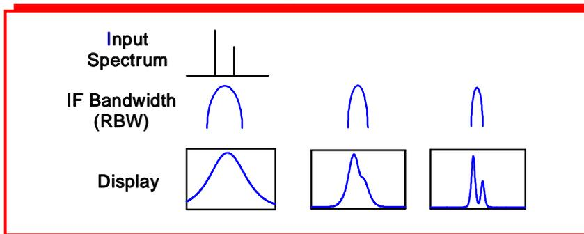
The IF filter is a bandpass filter which is used as the "window" for detecting signals. It's bandwidth is also called the resolution bandwidth (RBW) of the analyzer and can be changed via the front panel of the analyzer.
