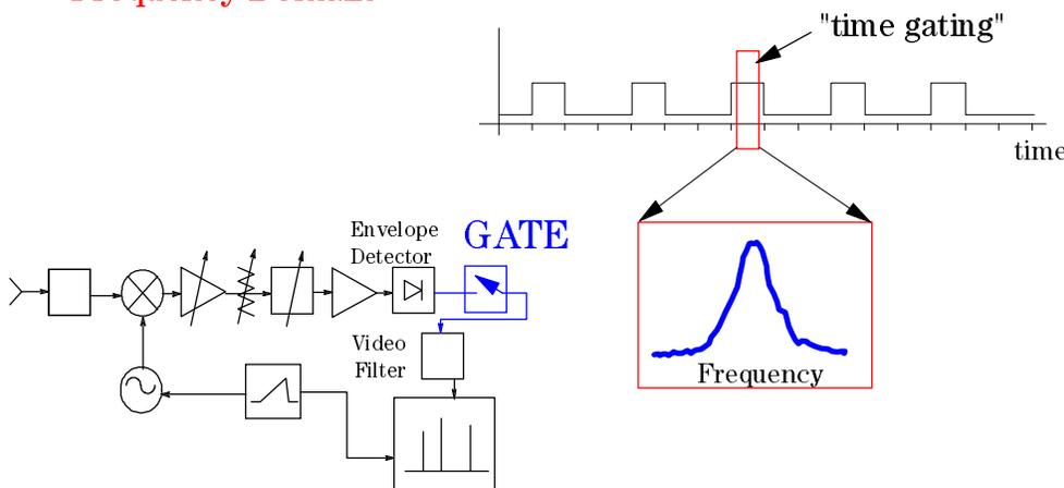
Time-gated, or time-selective spectrum analysis offers a solution to measurement difficulties in the time and frequency domains. Time gating permits precise yet flexible control of the point at which a time domain sweep begins, allowing the sweep to be centered over the desired timeslot. Any timeslot, or portion of a timeslot, may be examined at maximum time resolution.
