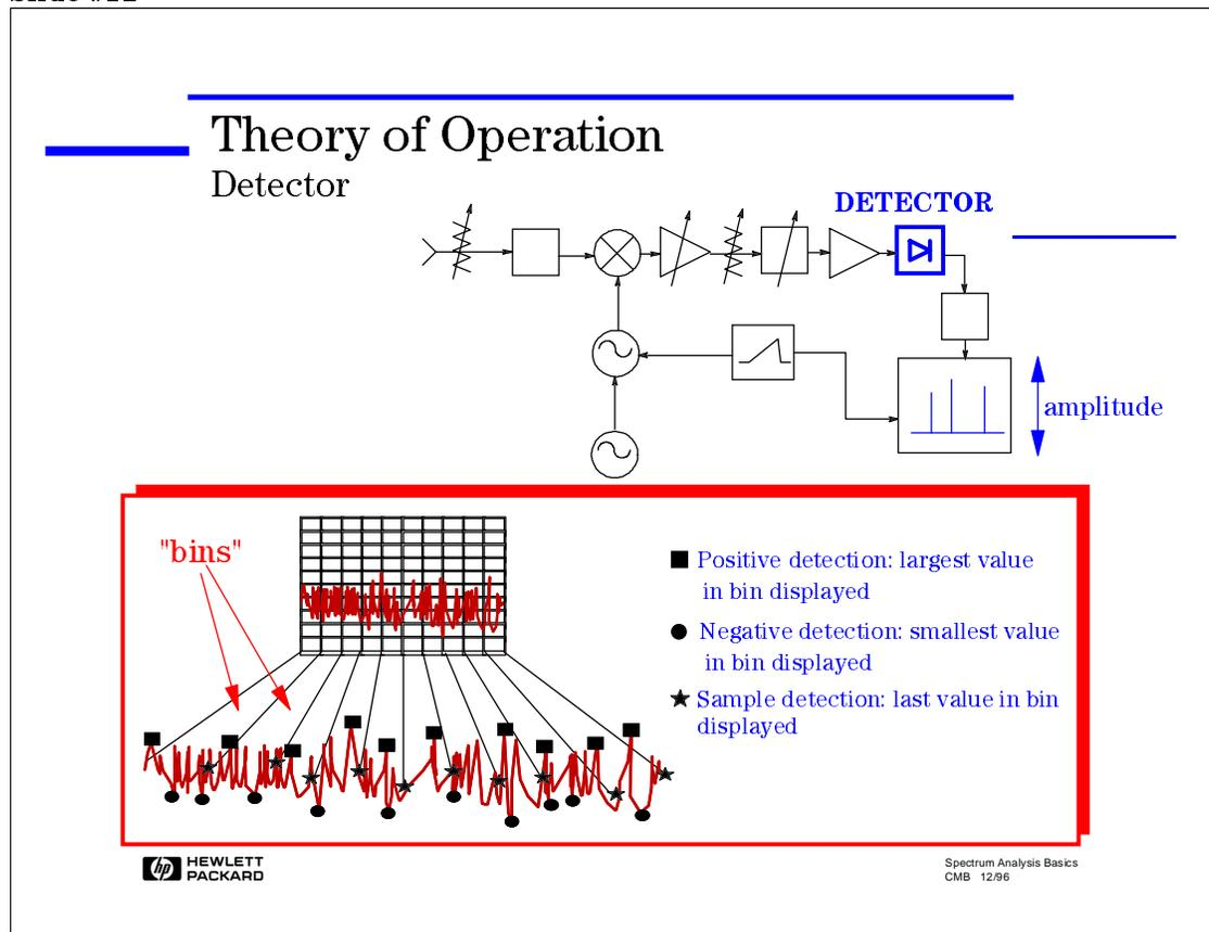
The analyzer must convert the IF signal to a baseband or video signal so it can be viewed on the instrument's display. This is accomplished with an envelope detector which then deflects the CRT beam on the y-axis, or amplitude axis.
