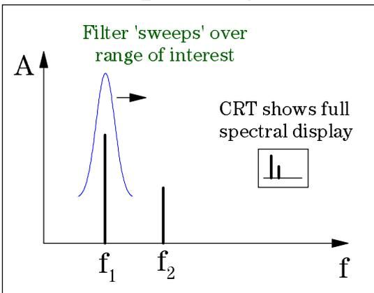
The diagram shows a graph with Amplitude (A) on the vertical axis and Frequency (f) on the horizontal axis. A blue curve represents the filter's response, which is sweeping across a range of interest between frequencies  $f_1$  and  $f_2$ . A peak in the curve is shown with an arrow pointing to the right. To the right of the graph, a small inset shows a CRT display with a full spectral display, represented by two vertical bars of different heights.
