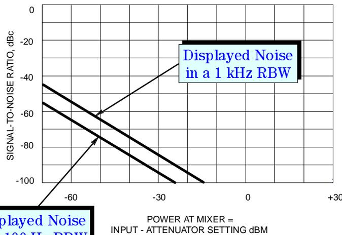
On page 48, we plotted the signal-to-distortion curves. This graph is actually called a dynamic range graph, and just as we plotted distortion products as a function of mixer power, we can also plot *signal-to-noise ratio* (SNR) as a function of mixer power.
