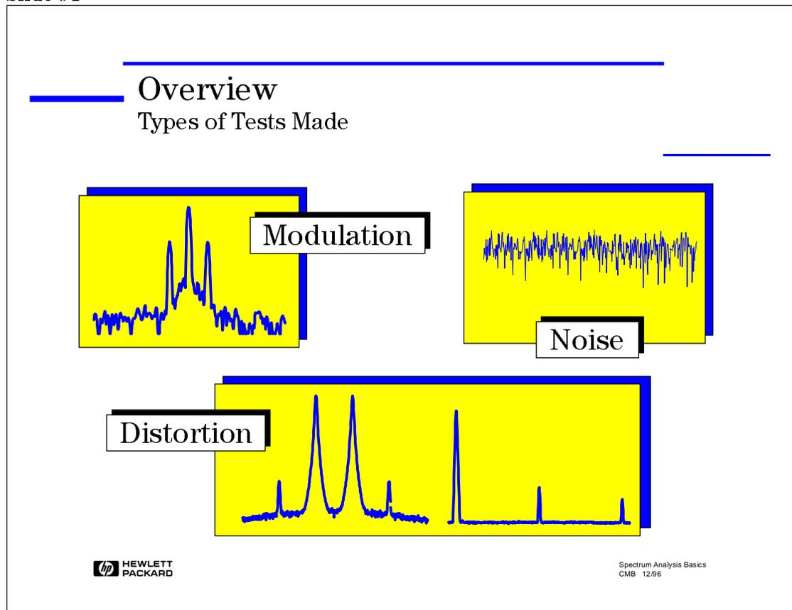
The most common spectrum analyzer measurements are: modulation, distortion, and noise.
