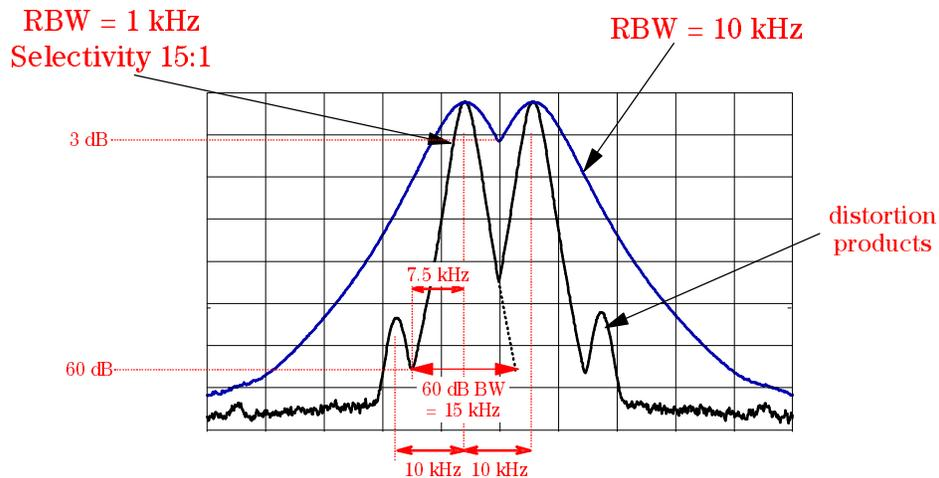
For example, say we are doing a two-tone test where the signals are separated by 10 kHz. With a 10 kHz RBW, resolution of the equal amplitude tones is not a problem, as we have seen. But the distortion products, which can be 50 dB down and 10 kHz away, could be buried.
