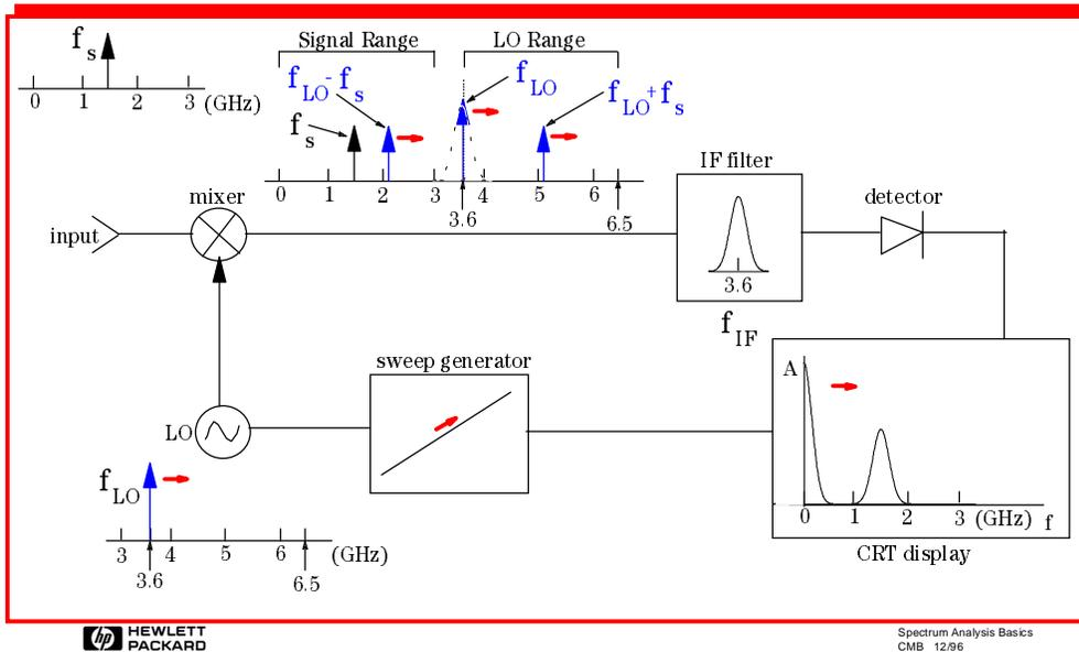
Let's see how these components work together to make a spectrum analyzer. Note that while the RF input attenuator, IF gain, and video filter are important components, they are not critical when describing how the analyzer works.
