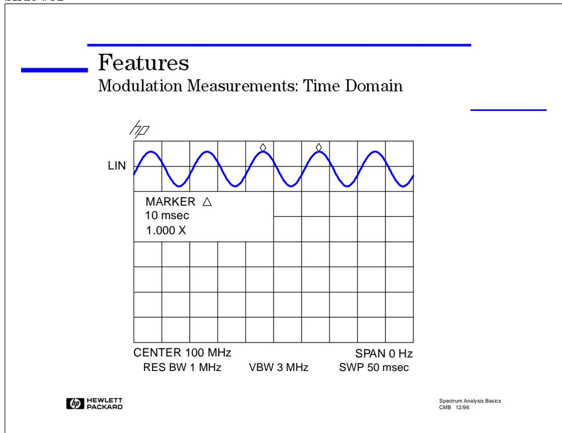
It was mentioned briefly that although a spectrum analyzer is primarily used to view signals in the frequency domain, it is also possible to use the spectrum analyzer to look at the time domain. This is done with a feature called zero-span. This is useful for determining modulation type or for demodulation.
