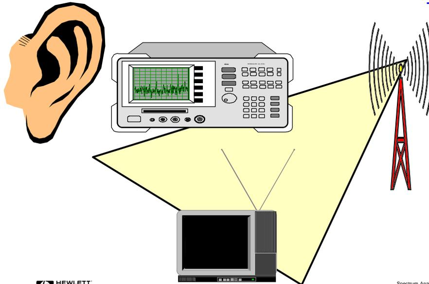
Most modern spectrum analyzers have available AM/FM detection with speakers. The built-in AM/FM detectors with speaker allow you to hear the modulation. In other words, they allow you to hear the source of interference as well as see it, for faster identification of interfering signals in communication networks, etc.
