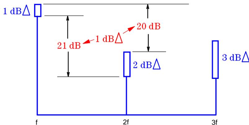
Most distortion measurements are made relative to the fundamental signals (the carrier or two-tones). When the fundamental power is decreased 1 dB, the second-order distortion decreases by 2 dB, but relative to the fundamental, the second-order distortion decreases 1 dB. There is a one-for-one *relative* relationship between the fundamental and second-order distortion.
