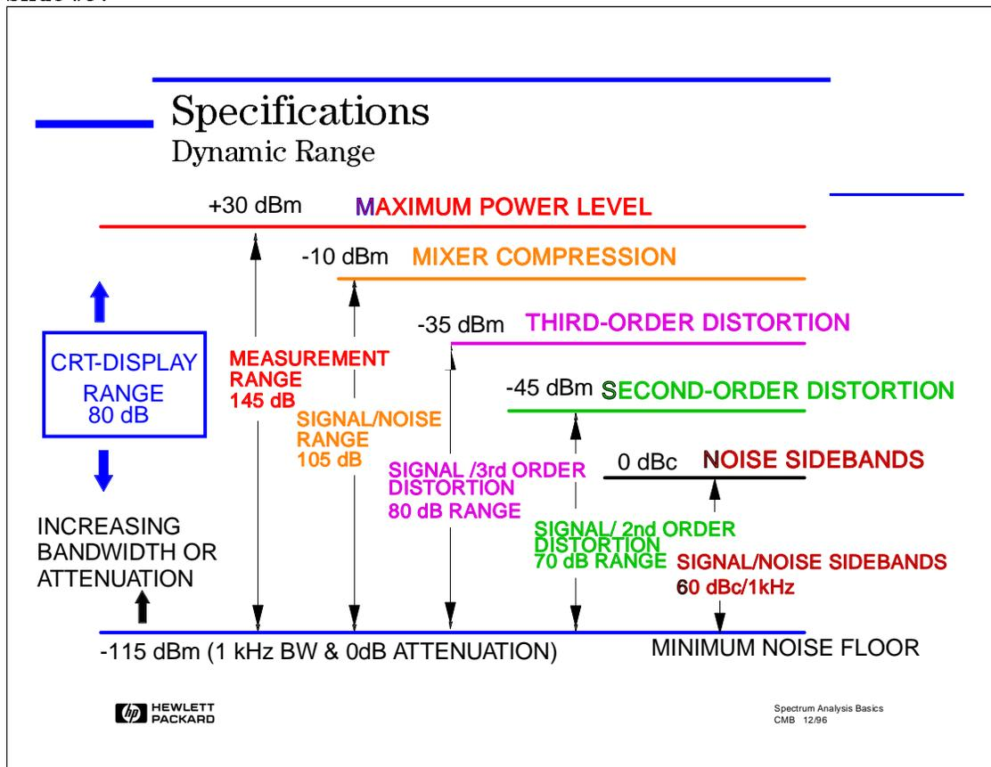
There are several ranges associated with the spectrum analyzer. Typically the term "dynamic range" only refers to the ability to measure two signals *at the same time*.
