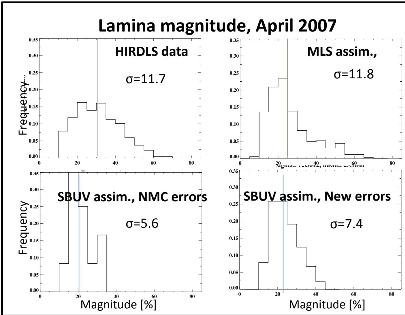
PDFs of (Max ozone - Min)/Max [%] for each identified lamina
