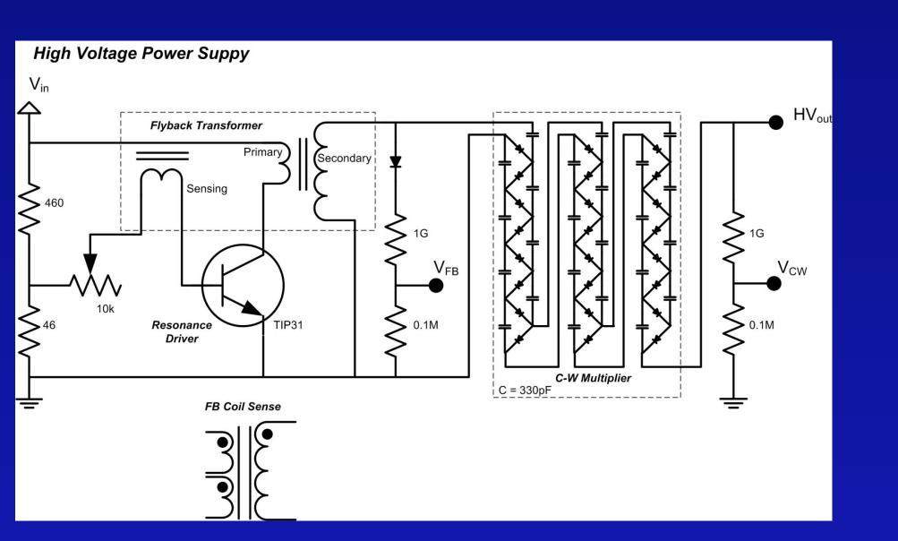
This circuit uses a resonant driven flyback transformer to pump a Cockcroft-Walton (1932) voltage multiplier. The key property of the multiplier is that voltage drops rapidly as current flows. This makes the generator a very sensitive conductivity meter.
