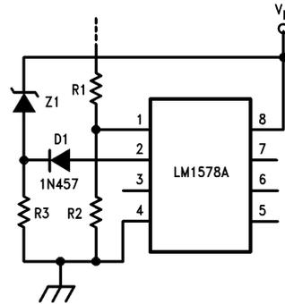
FIGURE 8. Under-Voltage Lockout
