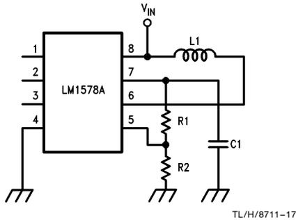
FIGURE 4. Current Limit Transient Suppressor, Ground Referred
