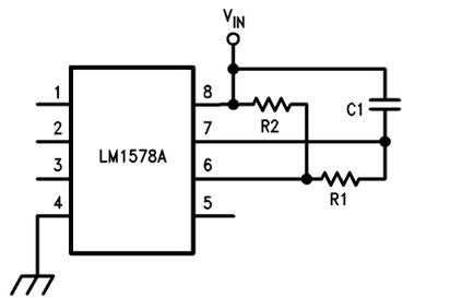
FIGURE 5. Current Limit Transient Suppressor,  $V_{in}$  Referred
