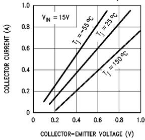
**Emitter Saturation Voltage (Sourcing Current, Collector at V<sub>IN</sub>)**
