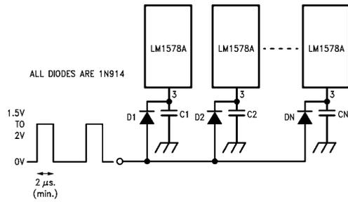
FIGURE 13. Synchronizing Devices
