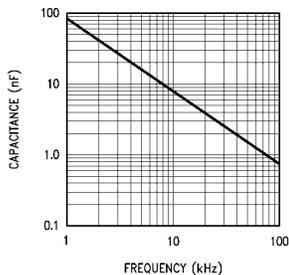
FIGURE 1. Value of Timing Capacitor vs Oscillator Frequency
