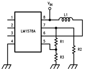
FIGURE 6. Current Limit Sense Voltage Multiplication, Ground Referred
