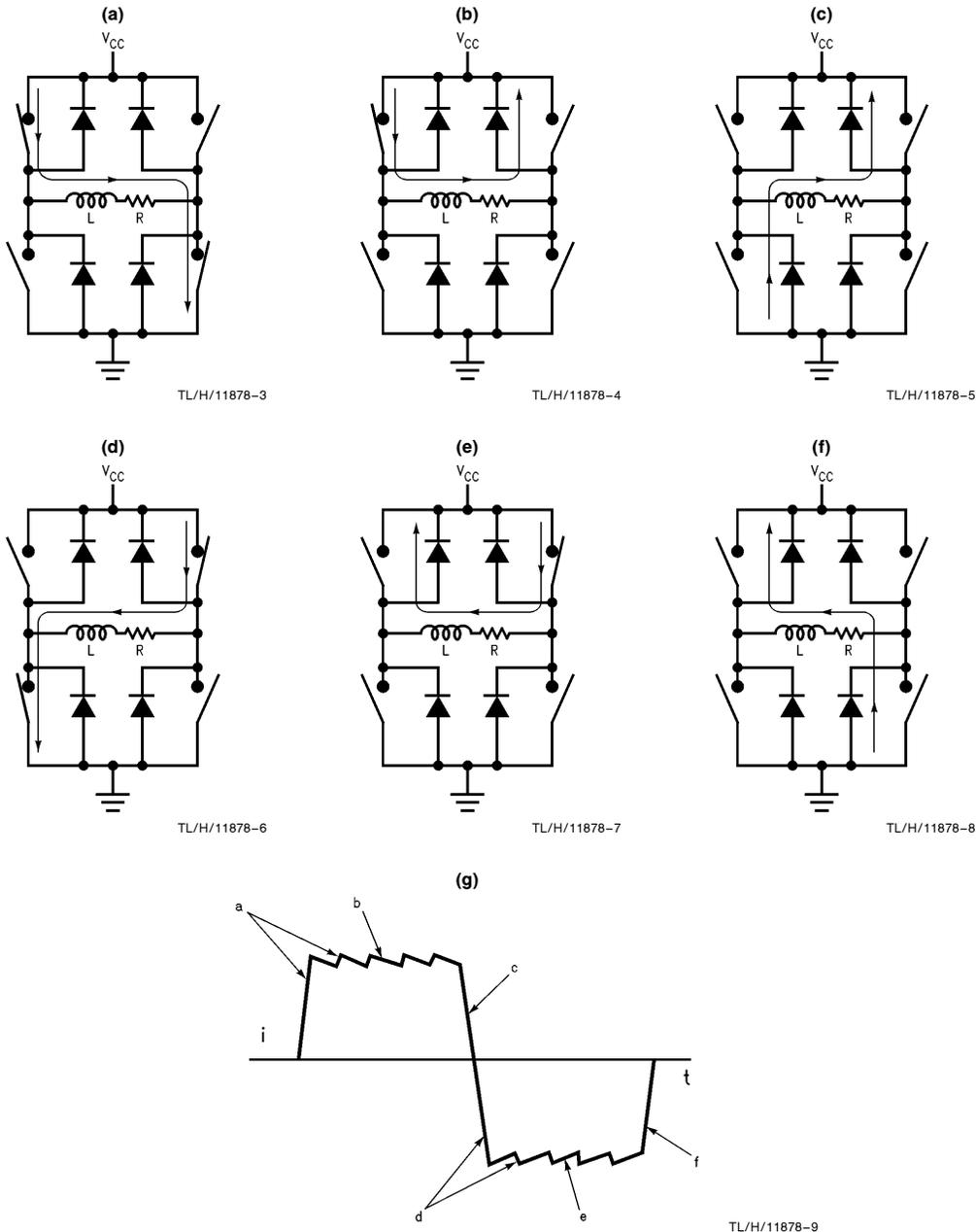
**FIGURE 1. Chopper Amplifier Chopping States: Full  $V_{CC}$  Applied Across the Winding (a) and (d), Shorted Winding (b) and (e), Winding Current Decays During a Change in the Direction of the Winding Current (c) and (f), and the Chopped Winding Current (g)**
