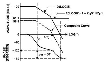
Figure 8-6. Bode Plot of Stability Equation
