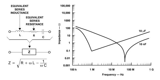
Figure 17–16. Capacitor Self Resonance
