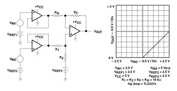
Figure A–18. Simplified High-Precision Differential Amplifier
