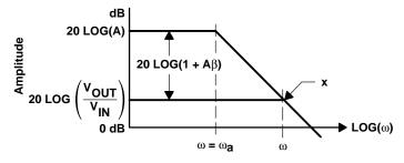
Figure 5-14. When Equation 5-12 has a Single Pole
