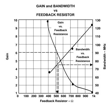
Figure 8–7. Plot of CFA RF, G, and BW
