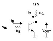
Figure 2–14. Saturated Transistor Circuit
