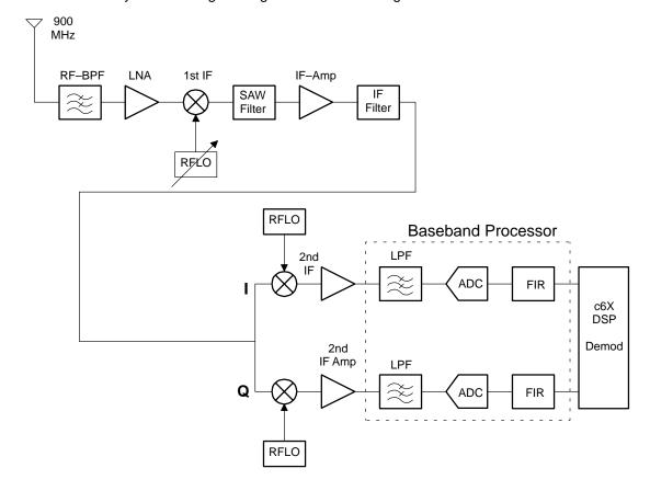
Figure 13–2. An Implementation of a Software-Configurable Dual-IF Receiver
