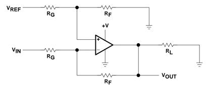
Figure 4-5. Inverting Op Amp
