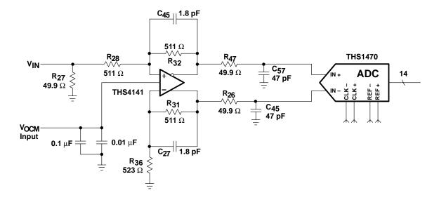
Figure 13-11. Single-Ended to Differential Output Drive Circuit
