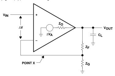
Figure 7-8. Capacitively-Loaded Op Amp
