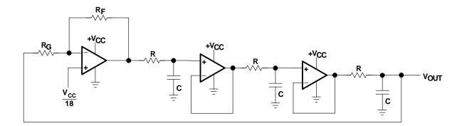
Figure A-42. Buffered Phase Shift Oscillator
