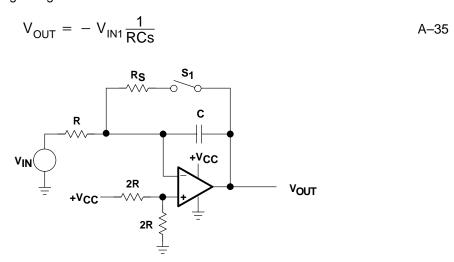
Figure A–30. Inverting Integrator with Mechanical Reset
