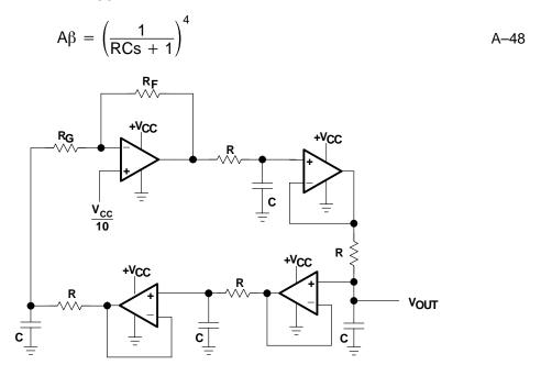
Figure A-43. Bubba Oscillator
