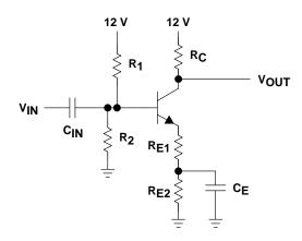
Figure 2–15. Transistor Amplifier
