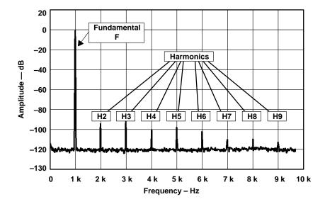
Figure 14-6. Total Harmonic Distortion
