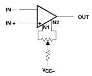
Figure 11–2. Offset Voltage Adjust
