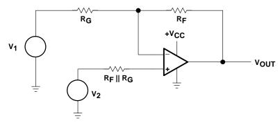
Figure 18–2. Noninverting Op Amp
