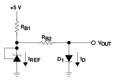
Figure 12–12. Reference and Transducer Bias Circuit
