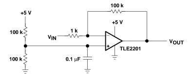
Figure 10–16. Improved TLC2201 Op Amp Circuit
