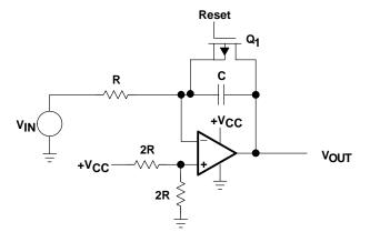
Figure A-31. Inverting Integrator with Electronic Reset
