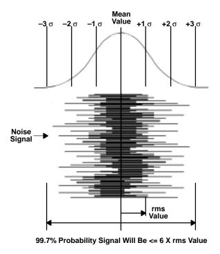
Figure 10–1. Gaussian Distribution of Noise Energy
