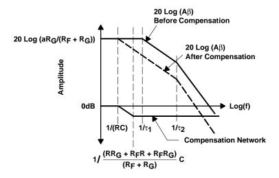
Figure 7-21. Bode Plot of Lead-Lag Compensated Op Amp
