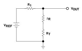
Figure 12-4. Voltage Divider Circuit for a Resistive Transducer
