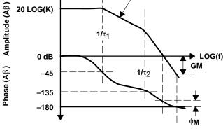
Figure 5-15. Magnitude and Phase Plot of Equation 5-14
