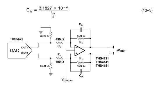
Figure 13-7. A Single-Pole Reconstruction Filter
