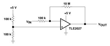
Figure 10-13. Split Supply Op Amp Circuit
