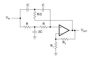
Figure 16-38. Active Twin-T Filter
