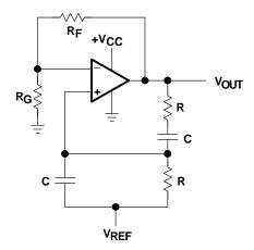
Figure A-37. Basic Wien Bridge Oscillator
