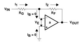
Figure 3–3. The Inverting Op Amp
