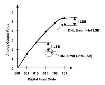
Figure 14-9. Differential Nonlinearity Error
