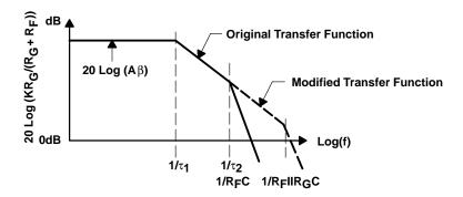
Figure 7–14. Lead-Compensation Bode Plot
