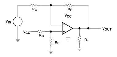
Figure 4-6. Inverting Op Amp With V<sub>CC</sub> Bias
