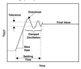
Figure 11–12. Settling Time
