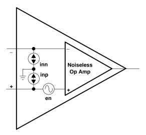
Figure 10-7. Op Amp Circuit Noise Model
