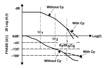
Figure 7-19. Compensated Attenuator Bode Plot
