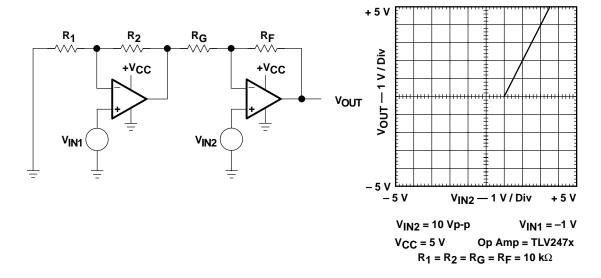
Figure A-15. High Input Impedance Differential Amplifier
