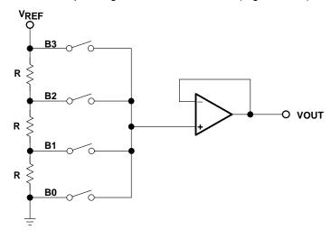
Figure 14-1. Resistor Ladder D/A Converter
