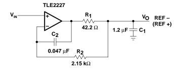
Figure 13-8. Voltage Reference Filter Circuit
