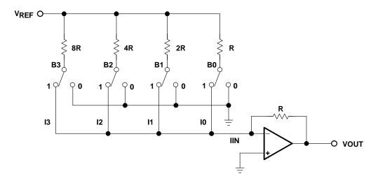
Figure 14–2. Binary Weighted D/A Converter
