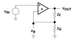
Figure 6-3. Noninverting Op Amp
