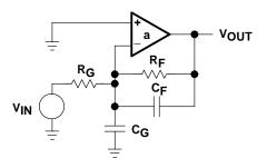
Figure 7–18. Compensated Attenuator Circuit
