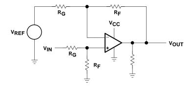
Figure 4-8. Noninverting Op Amp
