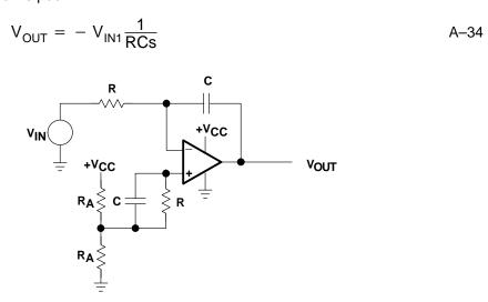
Figure A–29. Inverting Integrator with Drift Compensation
