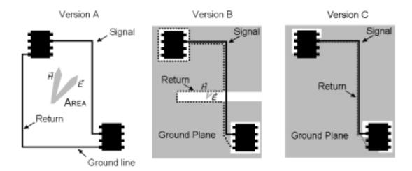
Figure 17–9. Loop and Slot Antenna Board Trace Layouts
