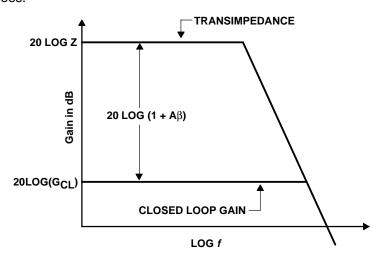
Figure 9-4. CFA Gain vs Frequency
