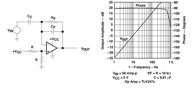
Figure A-36. Inverting Differentiator with Noise Filter
