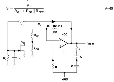
Figure A-39. Wien Bridge Oscillator with AGC
