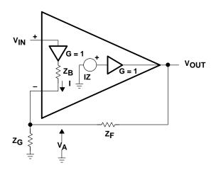
Figure 8-4. Noninverting CFA
