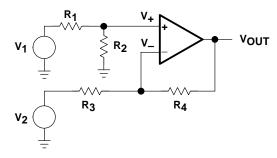
Figure 3-5. The Differential Amplifier
