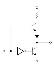
Figure 17–15. Logic Gate Output Structure
