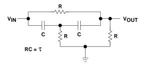
Figure 5-10. Band Reject Filter
