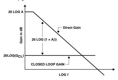
Figure 9–3. VFA Gain versus Frequency
