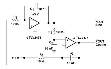
Figure 15–20. Quadrature Oscillator
