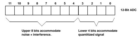
It follows from the above analysis that the GSM signal is 8 bits down, or 8 bits x 6 dB/bit = 48 dB down from the 1 V FSR of the ADC. The full-scale input power to an ADC having a  $50-\Omega$  termination can be calculated as:
