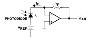
Figure 12–8. Photodiode Amplifier
