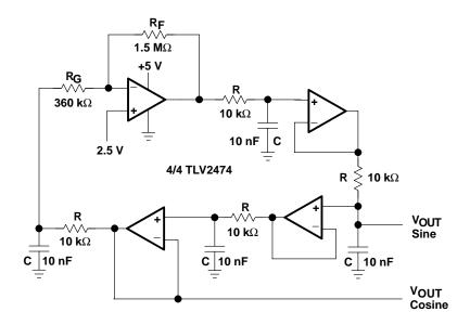
Figure 15-18. Bubba Oscillator
