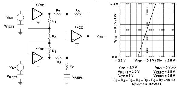
Figure A-17. High-Precision Differential Amplifier
