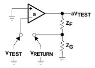
Figure 6-4. Open Loop Noninverting Op Amp
