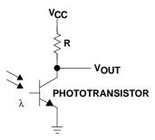
Figure 12–9. Phototransistor Amplifier
