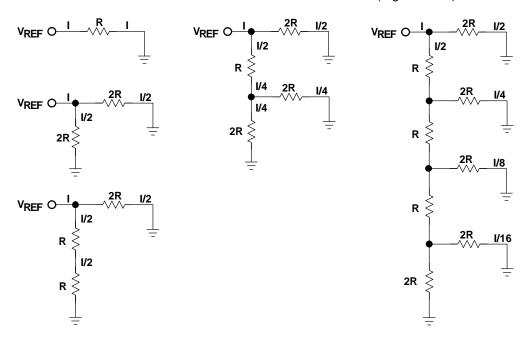
Figure 14–3. R/2R Resistor Array
