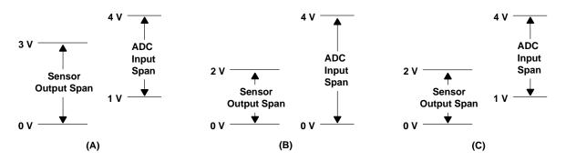
Figure 12-3. Example of Spans That Require Correction
