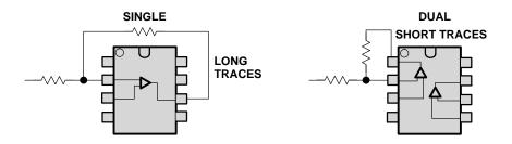
Figure 17–18. Trace Length for an Inverting Op Amp Stage
