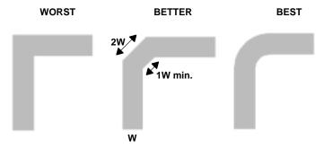
Figure 17-10. PCB Trace Corners
