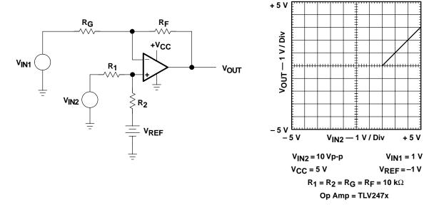
Figure A-14. Differential Amplifier with Bias Correction
