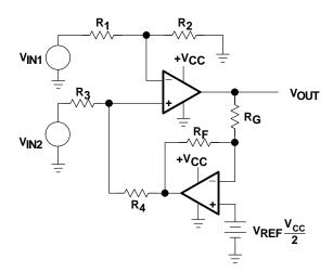
Figure A-19. Variable Gain Differential Amplifier
