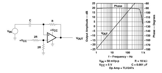
Figure A–35. Inverting Differentiator
