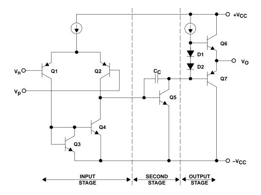
Figure 11-8. Figure 7. Simplified Op Amp Schematic
