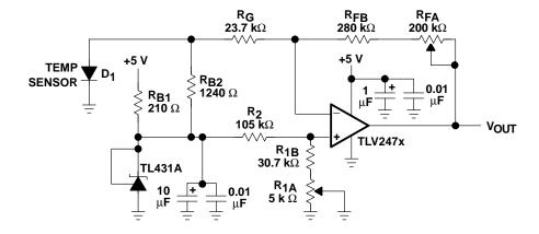
Figure 12-14. Final Analog Interface Circuit
