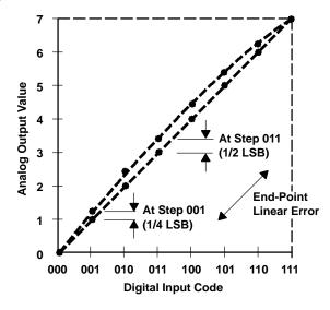
Figure 14–10. Integral Nonlinearity Error
