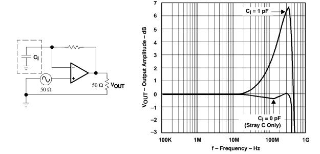
Figure 17–12. Effect of 1-pF Capacitance on Op Amp Inverting Input
