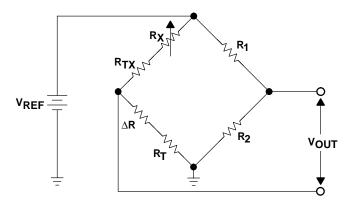
Figure 12-7. Wheatstone Bridge Circuit
