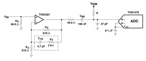
Figure 13-13. ADC Single-Ended Input Drive Circuit
