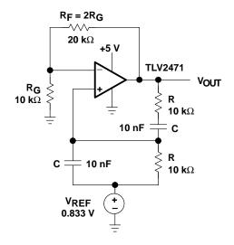
Figure 15–8. Final Wien Bridge Oscillator Circuit
