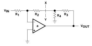
Figure 3–7. T Network in Feedback Loop
