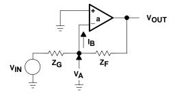
Figure 6-5. Inverting Op Amp
