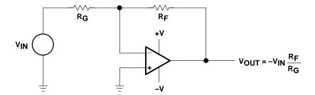
Figure 4-1. Split-Supply Op Amp Circuit
