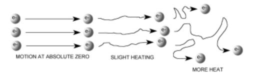
Figure 10-3. Thermal Noise
