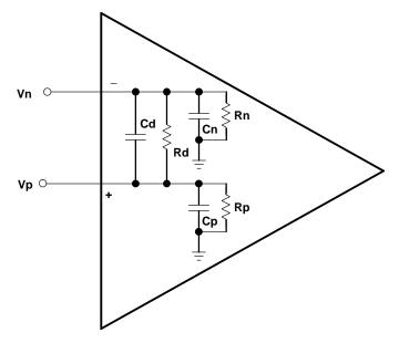
Figure 11-5. Input Parasitic Elements
