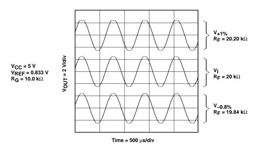
Figure 15-9. Wien Bridge Output Waveforms
