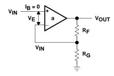
Figure 3–2. The Noninverting Op Amp
