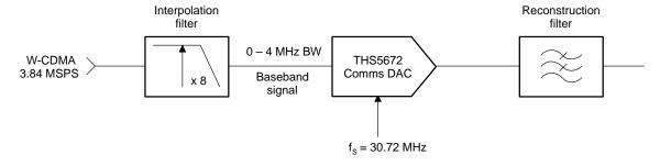
Figure 13-4. Communication DAC with Interpolation and Reconstruction Filters
