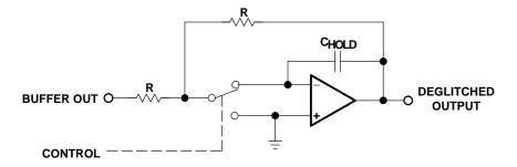
Figure 14-14. D/A Deglitch Circuit
