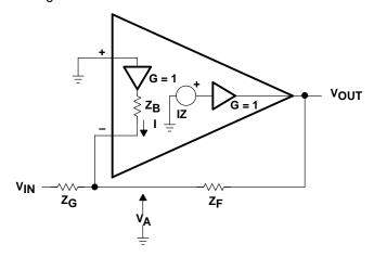
Figure 8-5. Inverting CFA
