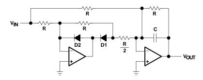
Figure 12-11. Active Full-Wave Rectifier and Filter
