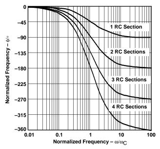
Figure 15-2. Phase Plot of RC Sections
