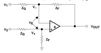
Figure 6-7. Differential Amplifier Circuit
