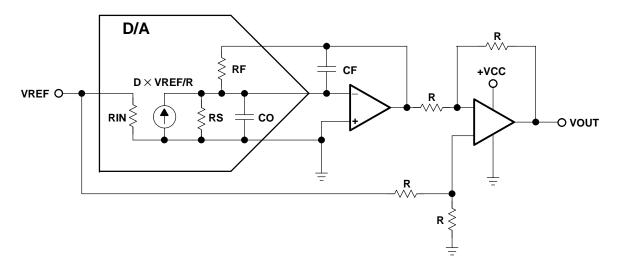
Figure 14–19. Single-Supply DAC Operation
