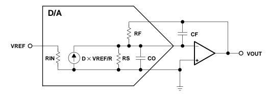
Figure 14-15. Compensating for CMOS DAC Output Capacitance
