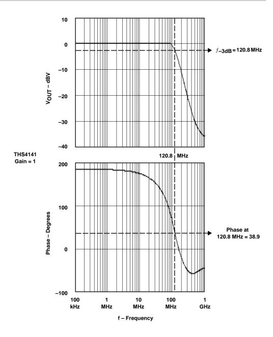
Figure 13–12. Differential Amplifier Closed-Loop Response
