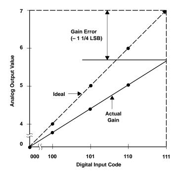
Figure 14-8. D/A Gain Error
