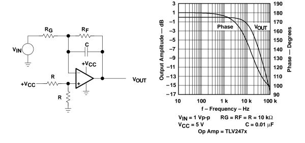
Figure A-32. Inverting Integrator with Resistive Reset
