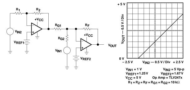
Figure A–16. High Common-Mode Range Differential Amplifier
