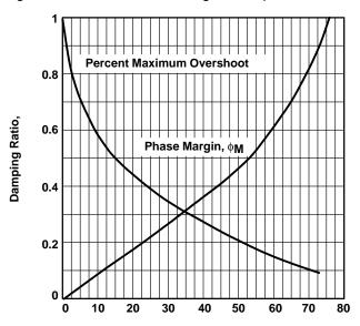
Figure 5–18. Phase Margin and Overshoot vs Damping Ratio
