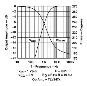
Figure A-22. Inverting AC Amplifier
