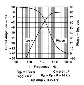
Figure A–23. Noninverting AC Amplifier
