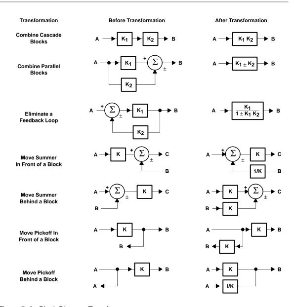
Figure 5-6. Block Diagram Transforms
