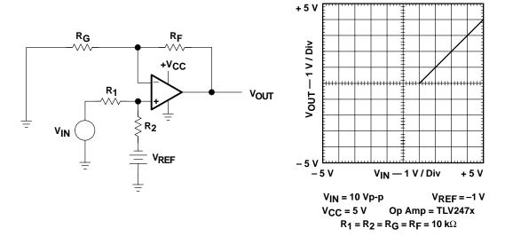
Figure A-10. Noninverting Op Amp with Noninverting Negative Reference
