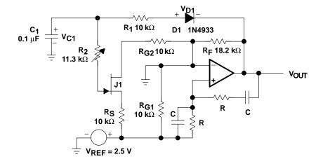
Figure 15-12. Wien Bridge Oscillator with AGC
