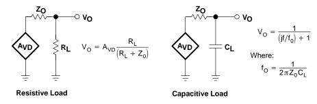
Figure 11-6. Effect of Output Impedance
