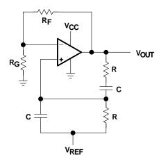
Figure 15–7. Wien Bridge Circuit Schematic
