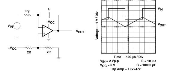
Figure A–27. Inverting Integrator
