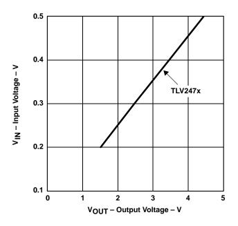
Figure 4-15. Case 2 Example Circuit Measured Transfer Curve
