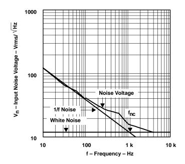
Figure 10-6. TLV2772 Op Amp Noise Characteristics
