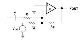
Figure 7-20. Lead-Lag Compensated Op Amp
