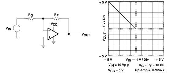
Figure A-4. Single-Supply Op Amp Circuit
