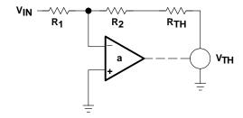
Figure 3–8. Thevenin's Theorem Applied to T Network
