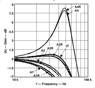
Figure 16–51. Differences in Q and f<sub>C</sub> in the Partial Filters of an Eighth-Order Butterworth Low-Pass Filter
