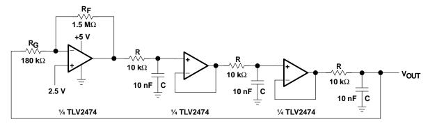
Figure 15–16. Phase Shift Oscillator, Buffered
