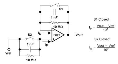
Figure 11–3. Test Circuit – I<sub>IB</sub>
