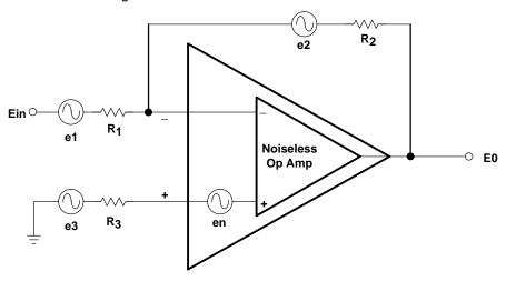
Figure 10-9. Inverting Op Amp Circuit Noise Model
