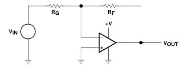
Figure 4-4. Single-Supply Op Amp Circuit
