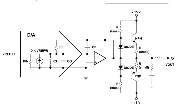
Figure 14–16. D/A Output Current Booster
