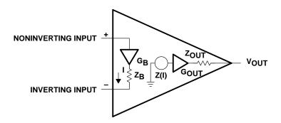
Figure 8-1. Current-Feedback Amplifier Model
