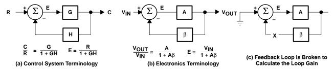
Figure 5–7. Comparison of Control and Electronic Canonical Feedback Systems
