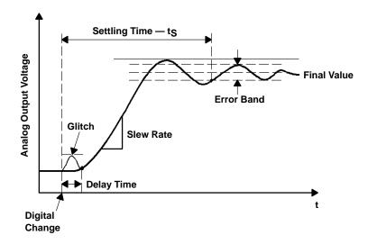
Figure 14-13. D/A Settling Time
