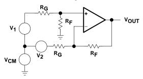
Figure 3-6. Differential Amplifier With Common-Mode Input Signal
