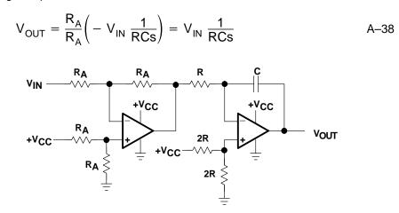
Figure A-33. Noninverting Integrator with Inverting Buffer
