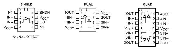
Figure 17–17. Common Op Amp Pinouts
