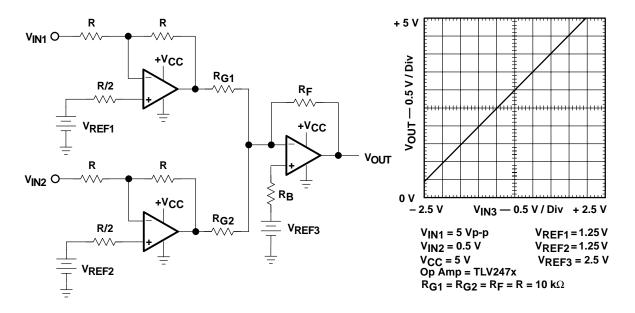
Figure A-26. Noninverting Summer with Buffers
