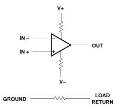
Figure 17-1. Op Amp Terminal Model
