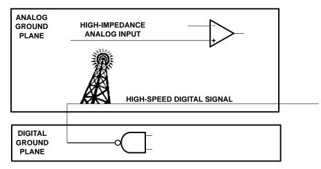
Figure 17–4. Broadcasting From PCB Traces
