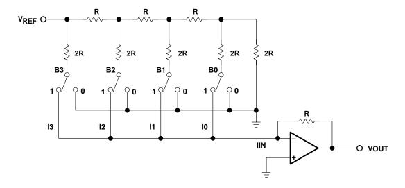
Figure 14–4. R/2R D/A Converter
