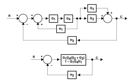
Figure 5-5. Multiloop Feedback System
