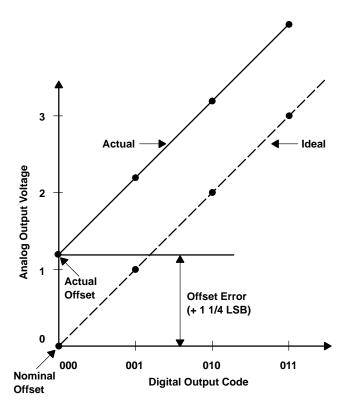
Figure 14-7. D/A Offset Error
