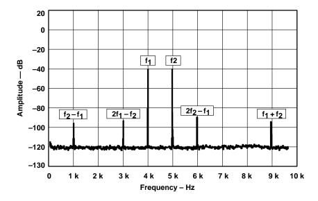
Figure 14-12. Intermodulation Distortion
