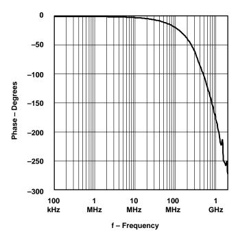
Figure 13-15. Phase vs Frequency for THS3201
