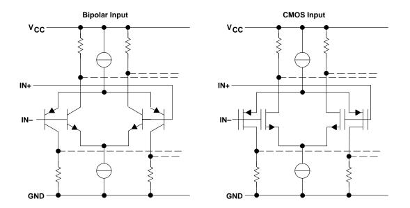
Figure 18-4. Input Circuit of an RRI Op Amp
