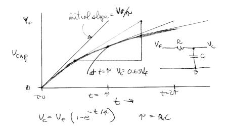
The input to the RC circuit is a step function going from 0 to Vf.
