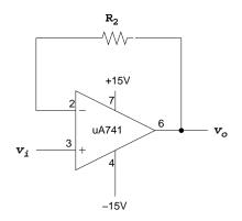
6. Replace the 741 with a 411 op amp. What is the DC output voltage now? Can you determine how much is due to input offset voltage and how much is due to input bias current? (Find  $I_B$  for the 411 from its spec sheet.)
