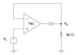
4. Substitute a 411 op amp for the 741. Compare the behavior of the two rectifiers at 2 kHz frequency. Why is the performance improved with the 411? (Hint: Look at the output of the op amp on the other trace.)
