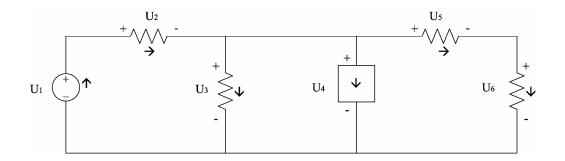
b. Sum the power values you obtained for elements  $U_2$  through  $U_6$ . Does this equal the value you calculated for the voltage source (with the opposite sign)? It should! Add them together, if they do not sum to zero then you have one or more errors in the table. As these values are related to each other, a mistake in one value could easily affect another. Check your work and check the power sum until you get it right. Your equation should look like this:
