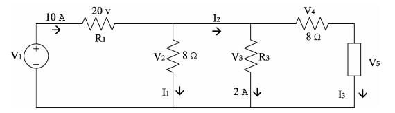
2. V<sub>1</sub> is providing 600 watts to the circuit shown above. Using KVL, KCL, Ohm's Law (OL), and Watt's Law (WL), label voltage reverences (+ and – polarity markers) for all circuit elements and solve for all unknown variables (V<sub>1</sub>, V<sub>2</sub>, V<sub>3</sub>, V<sub>4</sub>, V<sub>5</sub>, I<sub>1</sub>, I<sub>2</sub>, I<sub>3</sub>, R<sub>1</sub>, R<sub>3</sub>). Note which rule you are using for each calculation and perform a power balance check.
