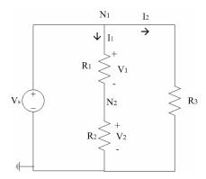
4. In the figure below, Vs = 10 v. With a multimeter we measure (w.r.t. Gnd) 4 v at  $N_1$  and 7 v at  $N_2$ . Find  $V_1$  and  $V_2$ .
