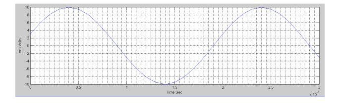
4. For the figure above, find the indicated values and express the function v(t) in equation form (*be careful to note that the units for time on this graph are in*  $10^{-5}$  seconds).
