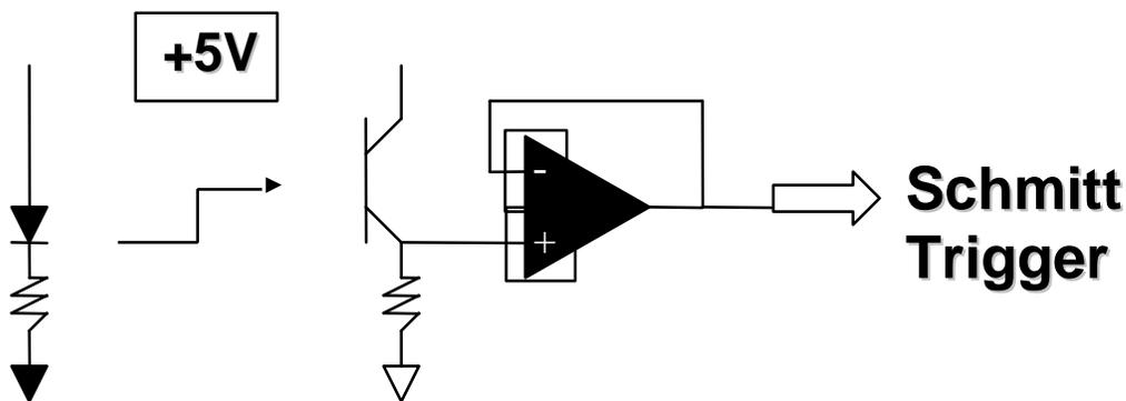
Figure 5: The White Line Sensor
