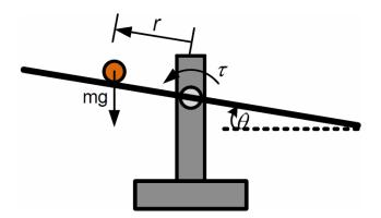
Assuming no slipping, one representation of the system are the state-space equations:
